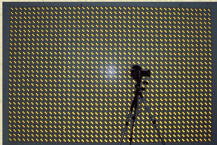
$$\begin{cases} x + \frac{l_1 X + l_2 Y + l_3 Z + l_4}{l_9 X + l_{10} Y + l_{11} Z + 1} = 0 \\ y + \frac{l_5 X + l_6 Y + l_7 Z + l_8}{l_9 X + l_{10} Y + l_{11} Z + 1} = 0 \end{cases}$$
