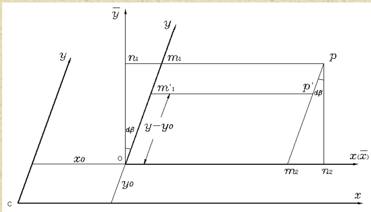
$$\begin{aligned} \delta y &= on_1 - om'_1 = om_1 \cdot \cos d\beta - om'_1 \\ &= (1 + ds)(y - y_0) \cdot \cos d\beta - (y - y_0) \\ &= [(1 + ds) \cdot \cos d\beta - 1](y - y_0) \end{aligned}$$
