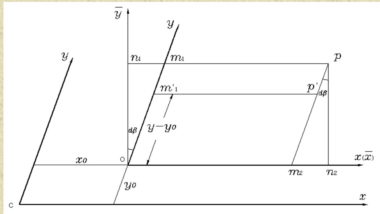
$$\begin{aligned} \delta x &= on_2 - om_2 = m_2 p \cdot \sin d\beta = om_1 \cdot \sin d\beta \\ &= (1 + ds)(y - y_0) \cdot \sin d\beta \end{aligned}$$
