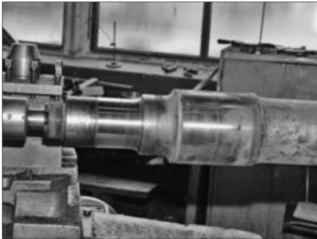
Figure 1. Damaged trunnion of a wagon axle
