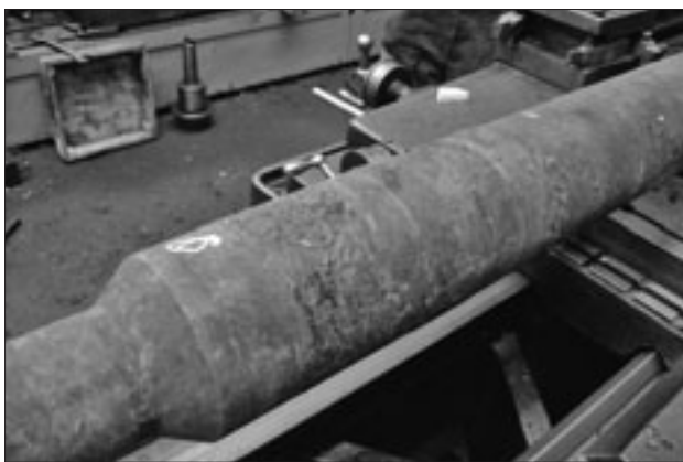
Figure 2. Damaged shaft of the screw press
