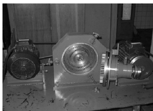
Figure 2. Disintegration type mill; productivity up to 150 kg per hour
