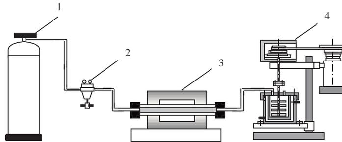
**Figure 1.** Mechanical alloying set-up: 1) Argon cylinder, 2) Manometer, 3) Tube furnace, 4) Attritor.
