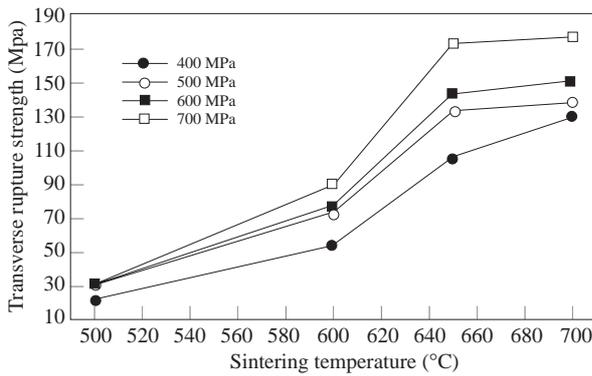
**Figure 6.** Relationship between sintering temperature and transverse rupture strength.
