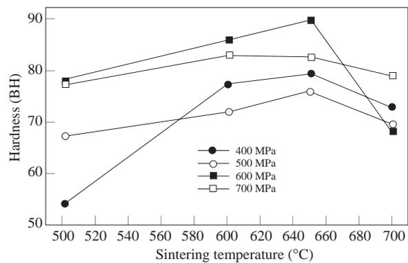
**Figure 7.** Effect of sintering temperature on hardness.
