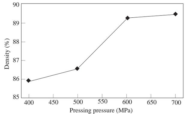
**Figure 4.** Relationship between compaction pressure and green density of samples.
