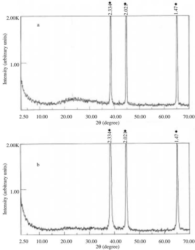
**Figure 3.** XRD result of the sample a) Before MA, b) After MA for 20 h.
