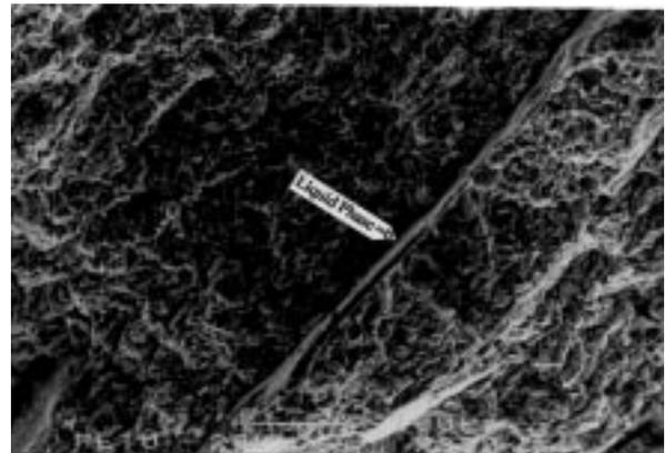
**Figure 10.** SEM micrograph of sample compacted at 600 MPa and sintered at 700°C for 5 h.
