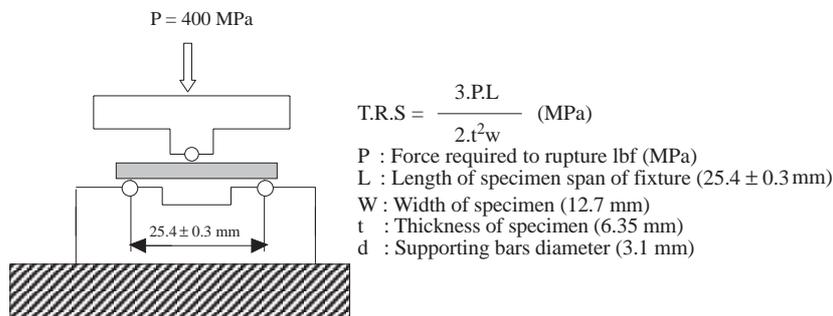
Figure 2. Transverse rupture test apparatus.
