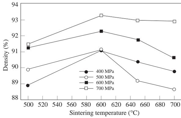
**Figure 5.** Relationship between sintering temperature and density of samples.
