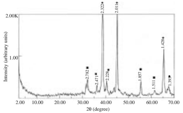
**Figure 8.** XRD result of the samples compacted at 600 MPa and sintered at 650°C. ♦ Al, ■  $Al_4C_3$ , ●  $Al_2O_3$ .
