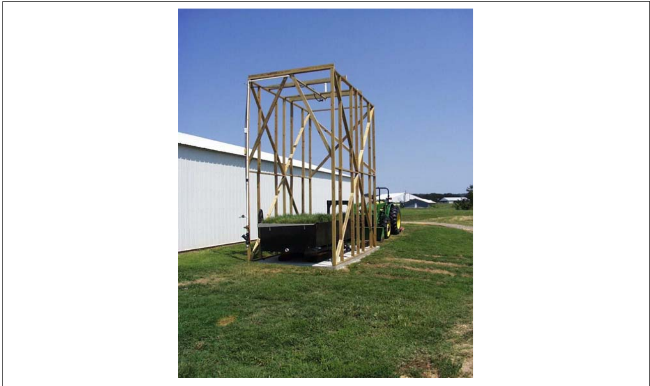
Figure 1. Picture of the variable slope box-plot located at the poultry farm on the University of Arkansas Agricultural Experiment Station, Fayetteville, Arkansas.
