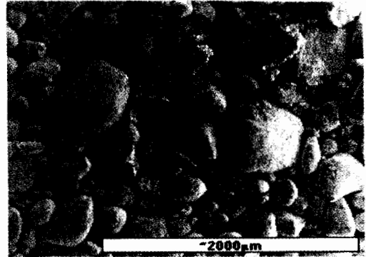
Fig. 3 Micrograph of corrosion product sample from the collection pipe of natural gas transport
