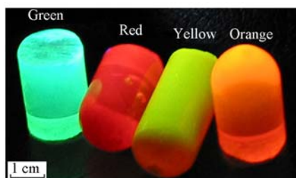
Fig. 6 Fluorescence image of four different CdTe-PS composite samples excited by an ultra-violet lamp
