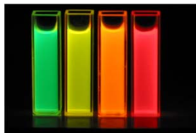
Fig. 1 Fluorescence images of differently sized CdTe nanocrystals prepared by hydrothermal technique
