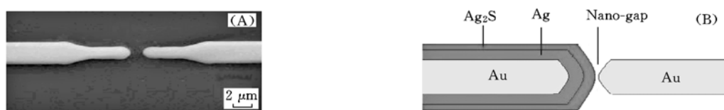
Fig. 1 SEM image of a pair of Au electrodes with a gap of 2 \mu\text{m} made by micro-fabricating method(A) and schematic diagram of a \text{Ag}_2\text{S} nano-switch(B)
