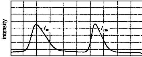
Fig 2 Measurement of standard waveform with \tau_{\omega 1/2}/\tau_{2\omega 1/2}= 1.429, \tau_{\omega 1/2}/\tau_{2\omega 1/4}= 1.004 图2 d=1\text{cm}, I_{\omega}=13\text{MW}/\text{cm}^2 时测量波形
