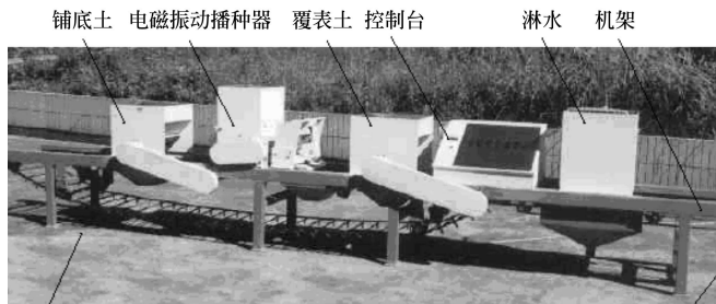
图2 2BZ-300型电磁振动式水稻育秧播种机 Fig.2 Electromagnetic vibrating rice nursing seedlings seeder of 2BZ-300 type
