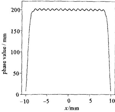
Fig. 3 Phase distribution with  $2\pi$  modulation frequency and 0.01nm modulation depth
