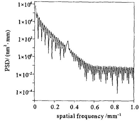
Fig. 4 PSD curve of the phase distribution with  $2\pi$
