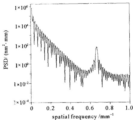
Fig. 9 PSD curve of the phase distribution with 0.01nm modulation depth
