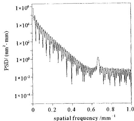
Fig. 10 PSD curve of the phase distribution with 0.0018nm modulation depth.
