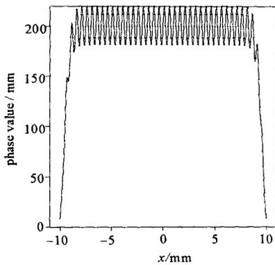
Fig. 7 Phase distribution with  $4\pi$  modulation frequency and 0.1nm modulation depth
