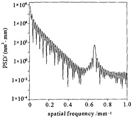
Fig. 5 PSD curve of the phase distribution with  $4\pi$  modulation frequency
