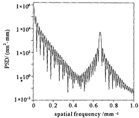
Fig. 8 PSD curve of the phase distribution with 0.1nm modulation depth
