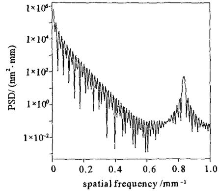
Fig. 6 PSD curve of the phase distribution with  $5\pi$  modulation frequency
