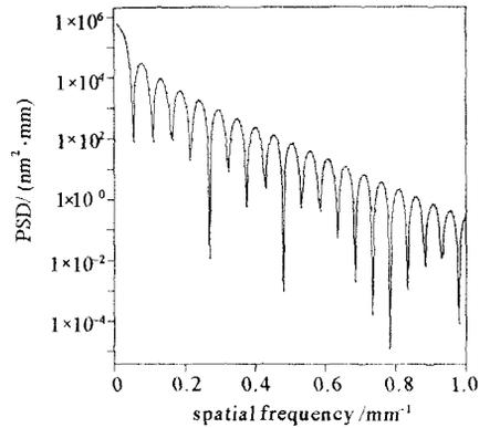
Fig. 2 PSD calculation result of the ideal wavefront
