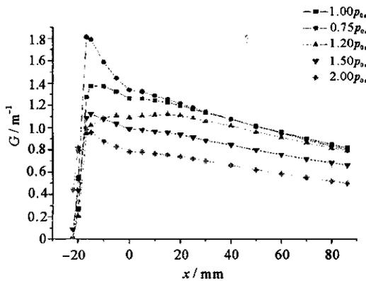
Fig. 5 Distribution of the average gain along  $x$  axis for different pressure of secondary flow
