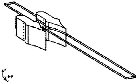
Fig. 1 COIL nozzle and computational zone
