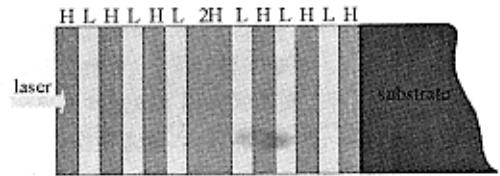
Fig. 2 Typical structure of one-cavity filter
