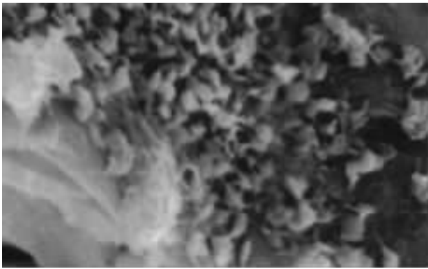
Fig 6 Platelet adhesion in TAXUS™ stent SEM × 100 图 6 TAXUS™ 支架血小板黏附
