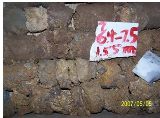
图 7 服务隧洞检查孔取芯照片 Fig.7 Photo of cores from examination hole in service tunnel
