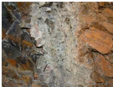
图 6 层间泥化夹层 Fig.6 Weak mud-stratum
