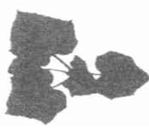
图 6 两次开运算 一次闭运算后消除噪声 Fig 6 Final binary image after morphological operation
