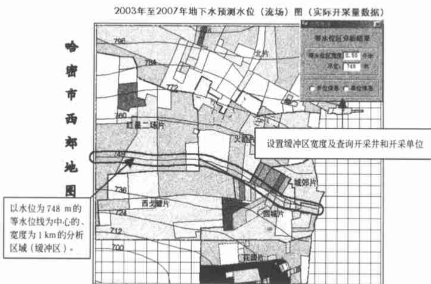
图 3 地下水流场图及缓冲区分析 Fig 3 Groundwater flow field graph and buffer analysis
