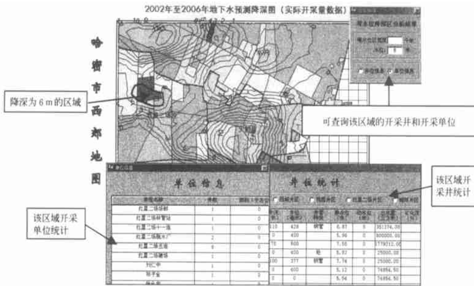
图 2 降深图及降深区域分析 Fig 2 Draw down graph and draw down analysis
