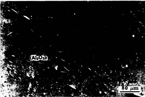
图 1 (Al 2 O 3 ) f /ZL 109 复合材料的 SEM 形貌 Fig.1 SEM photograph of the composite (Al 2 O 3 ) f /ZL 109
