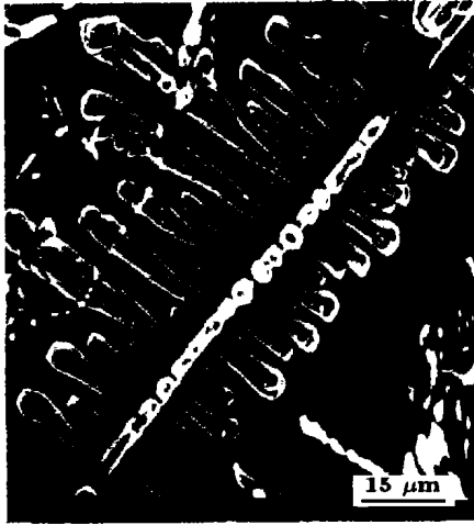
图 8 Ti-17Al-2C 合金中光滑枝晶状 \text{TiC} Fig.8 Smooth dendrite \text{TiC} in Ti-6Al-2C alloy
