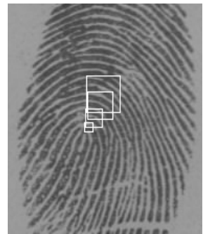
Fig.5 Corresponding relationship of the singularities detected with multilevel block sizes 图 5 各级分块尺寸下检测的奇异点的关联情况
