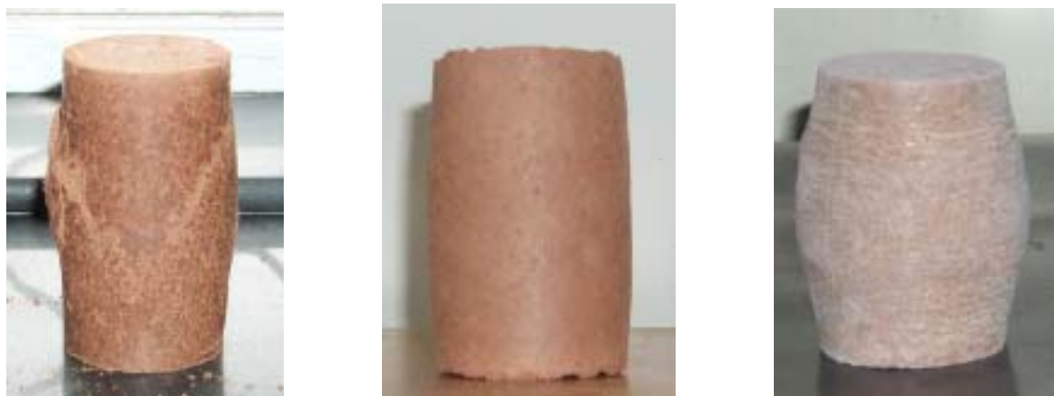
(a) 粉质粘土( \sigma_3=0.0 MPa, T=-4 ) (b) 粉质粘土( \sigma_3=6.0 MPa, T=-6 ) (c) 砂土( \sigma_3=8.0 MPa, T=-4 )
