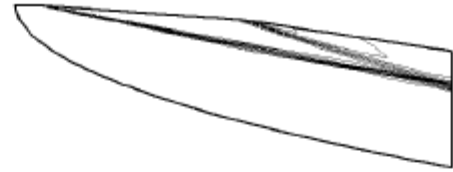
图 7 对称面的激波形状 Fig.7 Shock shape of symmetry plane
