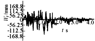
图 19 末端振动 Fig. 19 Experimental tip vibration of the manipulator
