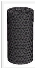
Figure 9: 3D mesh for image reconstruction with 858 nodes and 3208 tetrahedral elements.
