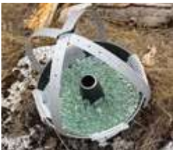
Close-up of a dust collector: pan, mesh, marbles and straps to keep birds from perching. Credit and Larger Version (/news/news_images.jsp?cntn_id=191381&org=NSF)
