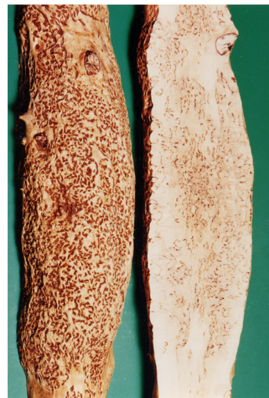
Figure 1. Curly birch timber – the surface of the trunk without bark (left) and longitudinal section of the trunk with decorative brown pattern (right)
