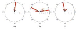
Fig. 8. Principal stress rose diagram (a) major principal stress (b) interim principal stress and (c) minor principal stress.
