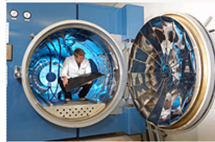
Researcher Chris Hurd in one of the autoclaves used to produce the carbon fibre structures
