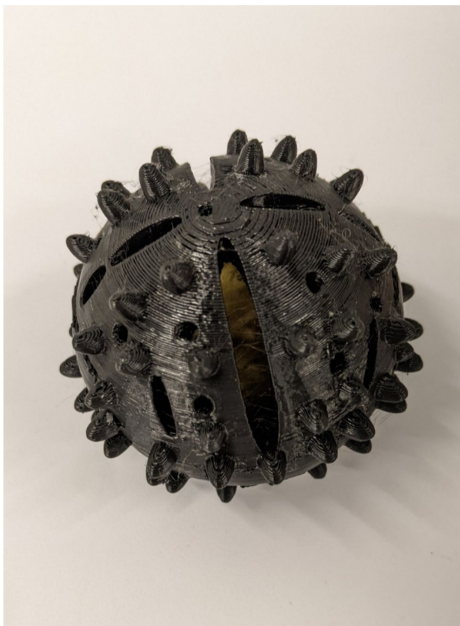
A CAD rendering and a 3D prototype of Baleena's microfiber-catching laundry ball.
