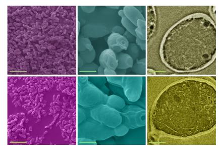
In this image, A control group of yeast cells (top row) is compared to yeast cells after they have accumulated lead from contaminated water (bottom row). Scanning electron microscope (SEM) images show, at left, an overview, and at center, a closer look at the yeast cells, and at right transmission electron microscope (TEM) images show an individual yeast cell.
