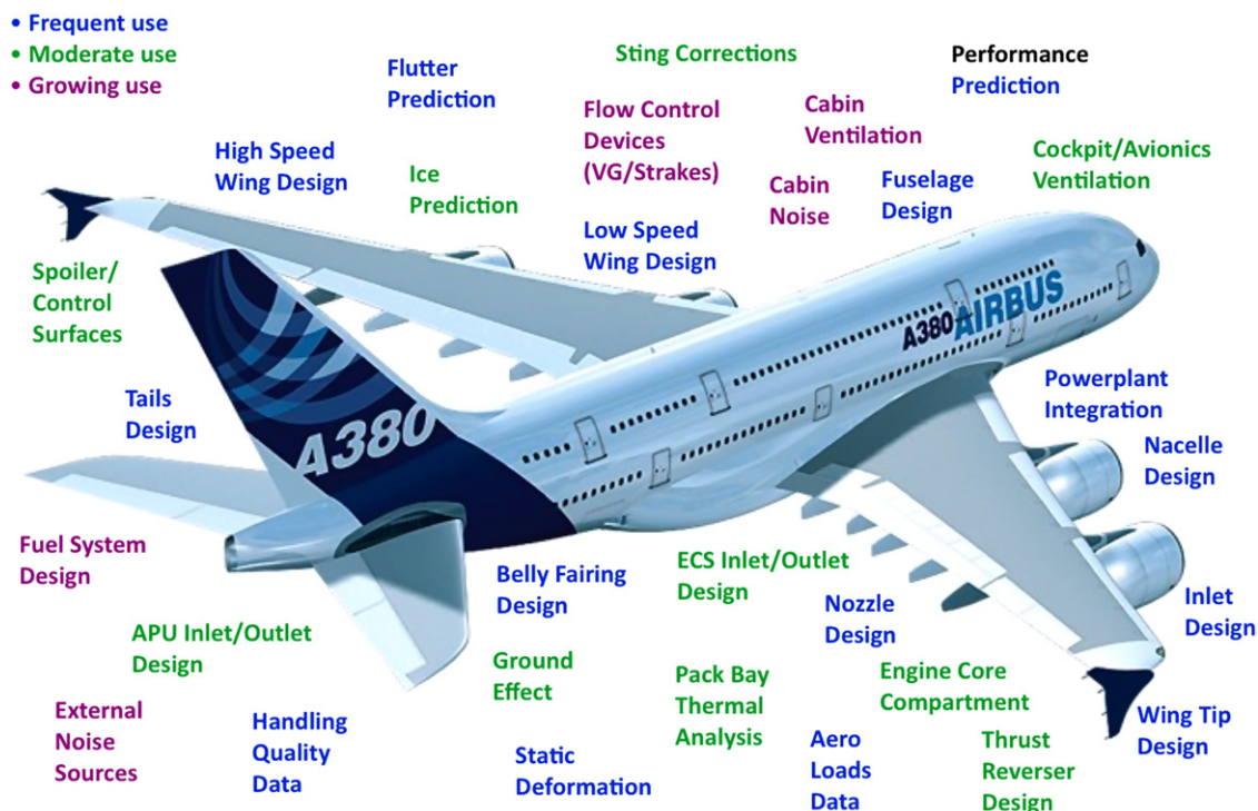
Fig. 4. Example of growing use of CFD in today's Airbus A380.
