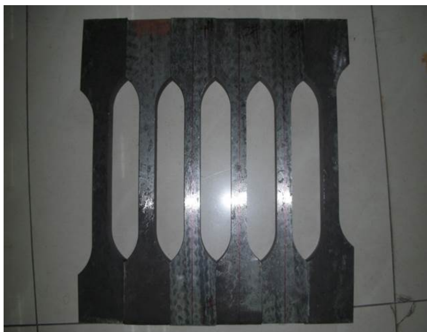
Figure 2. Practical specimen of Q225 under monotonic tensile tests
