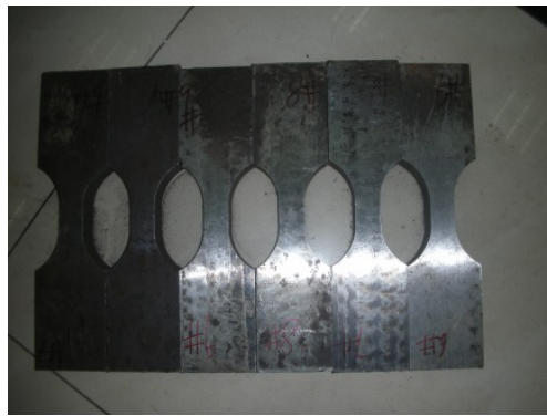
Figure 4. Practical specimen of Q225 under repeated loading tests
