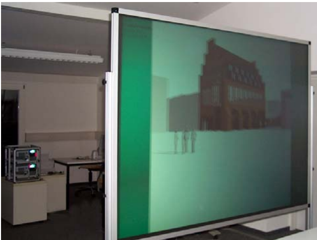
Figure 3: GeoWall. Projector rack and back projection screen
