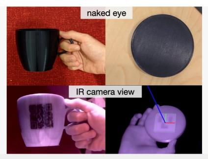
MIT scientists built a user interface that facilitates the integration of common tags (QR codes or ArUco markers used for augmented reality) with the object geometry to make them 3D printable as InfraredTags.
