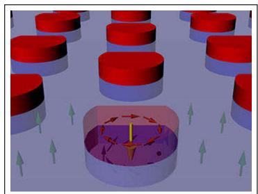
A magnetized cobalt disk (red) placed atop a thin cobaltpalladium film (light purple background) can be made to confer its own ringed configuration of magnetic moments (orange arrows) to the film below (purple arrows), creating a skyrmion in the film. The skyrmion, which is stable at room temperature, might be usable in computer memory systems.
