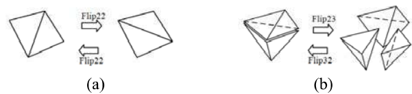
Figure 4. Flips are dynamic operations and make appropriate local updates in mesh data structure, a) flip22 in 2D, b) flip23 and flip32 in 3D.
