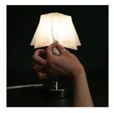
In this deformation-sensing lamp, the solid supports, textile lampshade, and sensing conductive pads are created as a single print.
