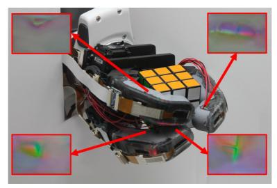
MIT researchers developed a soft-rigid robotic finger that incorporates powerful sensors along its entire length, enabling them to produce a robotic hand that could accurately identify objects after only one grasp.
