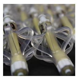
These new, soft actuators harnesses the power of instability to trigger instantaneous movement (photo courtesy of the Bertoldi Group)
