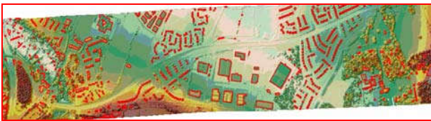
Figure 16: Extracted Building Boundaries
