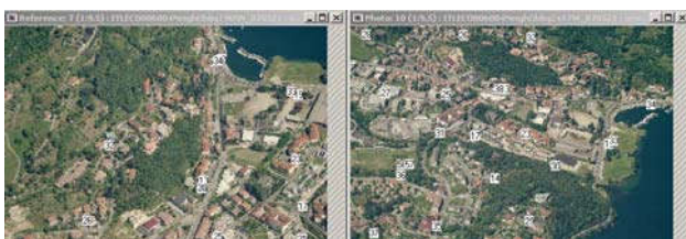
Figure 5. Oblique Image collected tie point, image are 90 degree direction (S-E) staggered. The interpretation of the images and the recognition of homologues point is not simple
