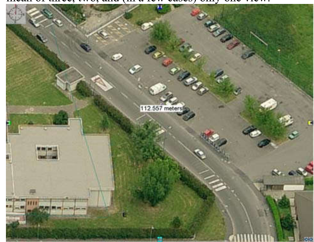
Figure 4. Direct measure of point elevation in oblique images realized in Pictometry EFS system
