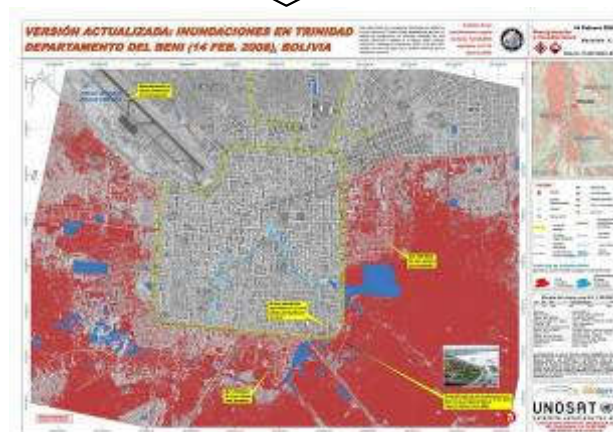
Fig. 12: Flooding in the urban area of Trinidad, TerraSAR(SL) /Radarsat radar images Source: TerraSAR-X; Radarsat, 1 m SpotLight (X-Band) resolution.- @UNOSAT2008
