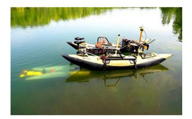
An underwater robot finds its way to a mobile docking station to recharge and upload data. <u>Credit and Larger Version (/discoveries/disc\_images.jsp?cntn\_id=301452&org=NSF)</u>
