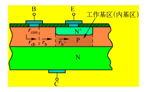
Large area bipolar transistors can have a very non-uniform current distribution due to the resistance of the base layer. Since the base current is applied through the thin base layer, there can be a significant series resistance in large devices.
