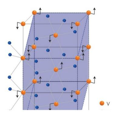
A schematic of the crystal structures in VO2, showing the motion of the vanadium (black arrows) with respect to the oxygen ions across the metal-insulator transition. VO2 acts like an insulator at low temperatures but like a metal at near room temperature.
