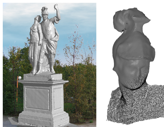
Figure 6: Rendered model (left), and rendering of the head and the corresponding triangulation (right)
