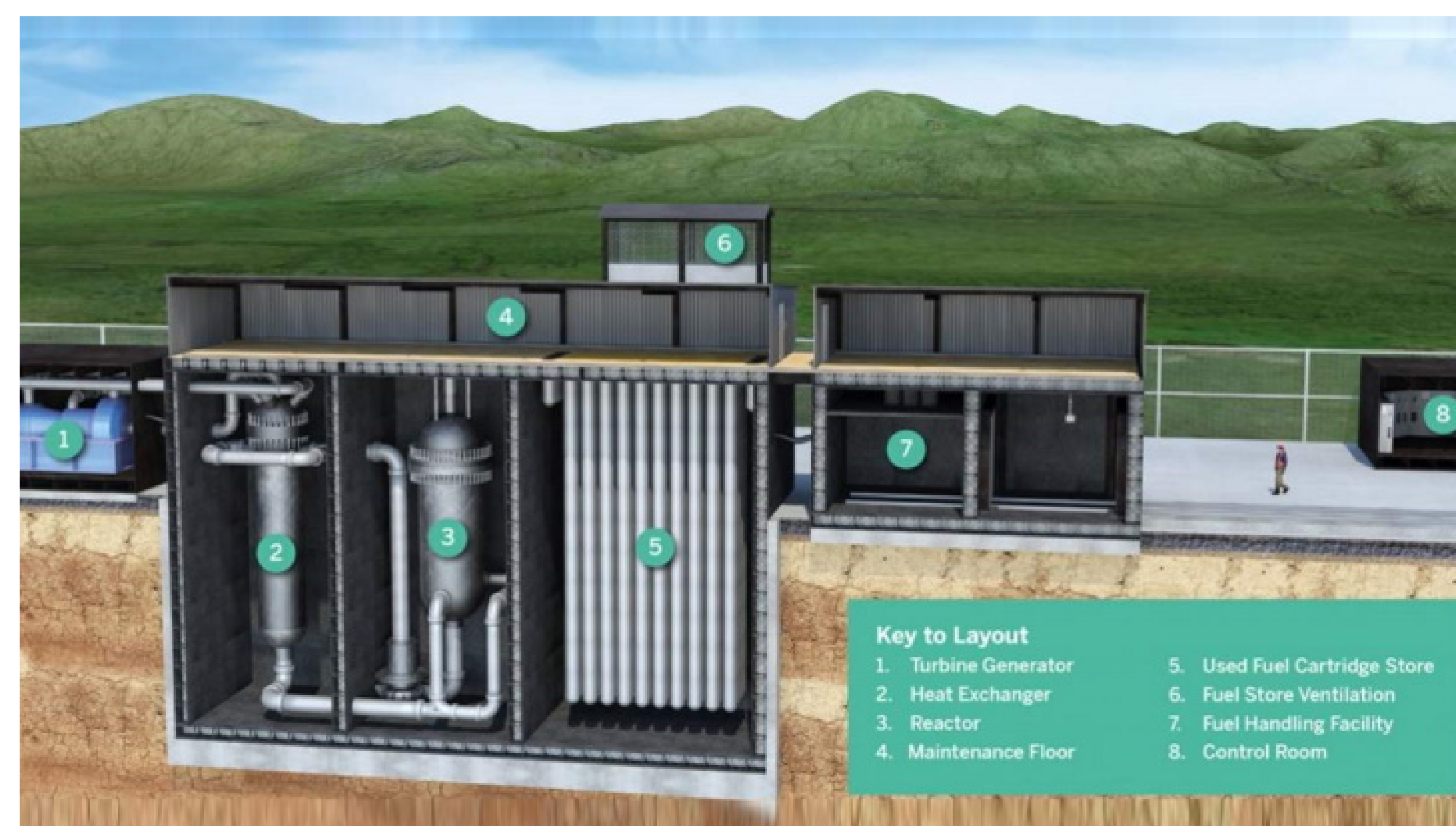
A cutaway of a plant based on the U-Battery reactor (Image: U-Battery)
