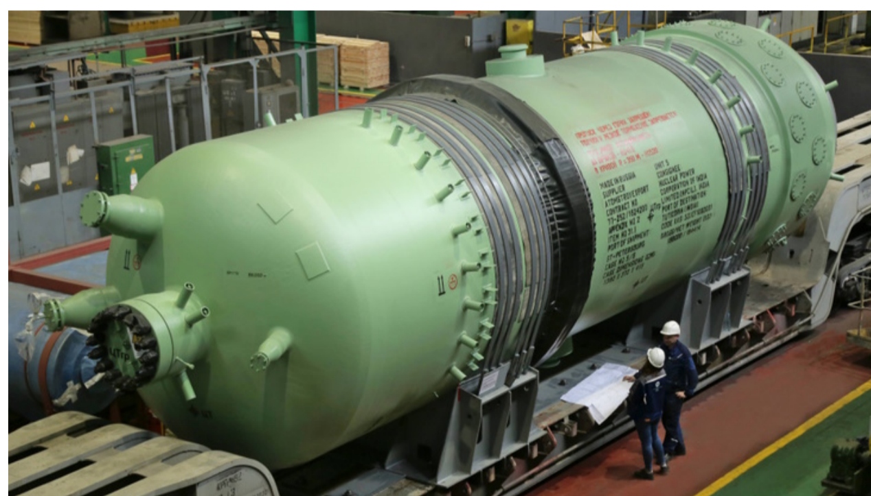
A pressuriser for Kudankulam 5, one of four VVER reactors currently under construction in Tamil Nadu, begins its journey of 17,000 km to the site on 4 April. The pressuriser, made by AEM-Technologies Izhora (part of Rosatom's machine-building division, Atomenergomash), weighs more than 187 tonnes and is about 14 metres in length (Image: AEM)
