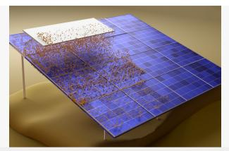
Dust that accumulates on solar panels is a major problem, but washing the panels uses huge amounts of water. MIT engineers have now developed a waterless cleaning method to remove dust on solar installations in water-limited regions, improving overall efficiency.
